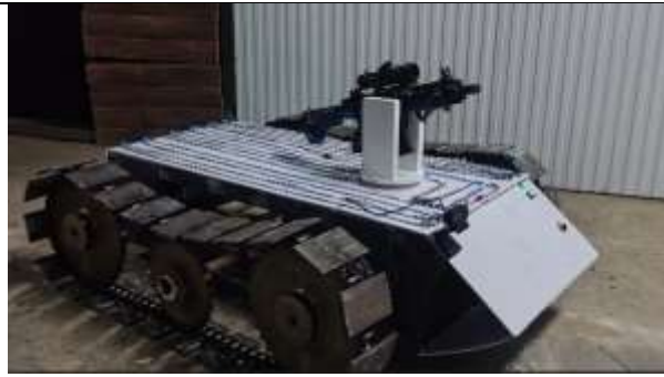
Figure 6- Experimental setup of the proposed autonomous ground robot during controlled field testing, showing tracked locomotion system, adaptive camouflage panel, and onboard sensing modules.
